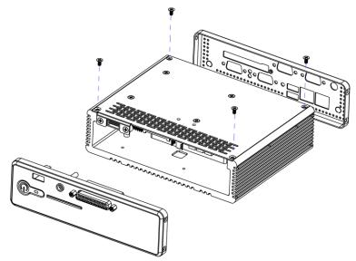
Step 2. Detach front & rear chassis, then remove 4 screws from the bottom side
