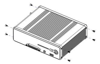
**Step 5.** Return & fasten 8 screws back to complete installation.
