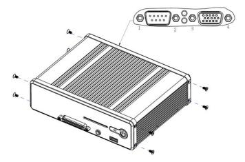
Step 1. Remove 8 screws from two sides, 4 screws from COM and VGA as displayed above, before you can remove the chassis cover.
