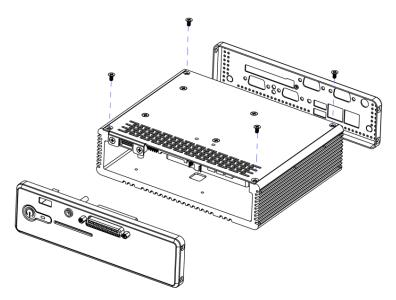
Step 4. Re-place the bottom cover, fasten with 4 screws to lock, then re-assemble the front/rear chassis
