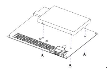
Step 3. Install HDD by means of 3 screws as shown above.
