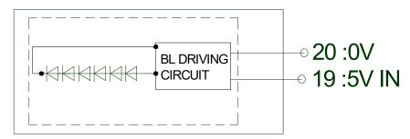
PIN20 is connected to PIN1(VSS) internally
