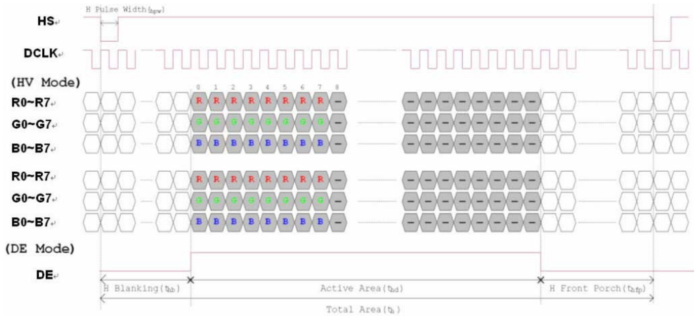
Figure 3.1 Horizontal input timing diagram
