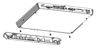
**Step 8.** Reassemble the rear chassis and fasten 3 screws to lock.
