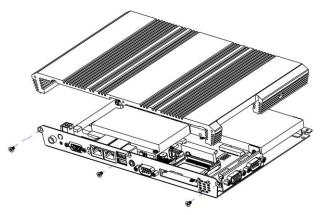
**Step 5-3.** Insert the HDD into the Drive Bay. Remember to properly seat the HDD so as to match screws and HDD holes.
