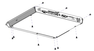
**Step 1.** Remove 10 screws from the case, and 4 screws from COM and VGA ports.
