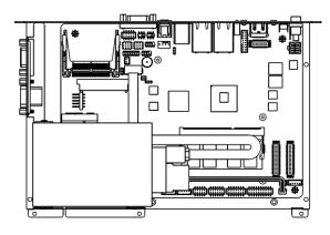
**Step 5-2.** Place HDD and SATA cable as shown above for a proper installation of the HDD.
