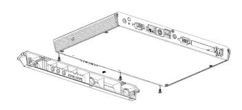
Step 8. Reassemble the rear chassis and fasten 3 screws to lock.
