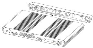
**Step 1.** Remove 10 screws from the case, and 4 screws **Step 2.** Remove the rear chassis. from COM and VGA ports.
