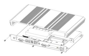
Step 6. Reassemble the top chassis and fasten with 3 screws.
