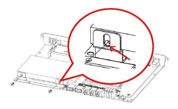
Step 5-3. Insert the HDD into the Drive Bay. Remember to properly seat the HDD so as to match screws and HDD holes.
