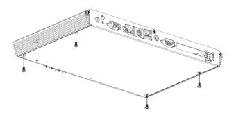
Step 7. Fasten 4 screws from the bottom chassis.
