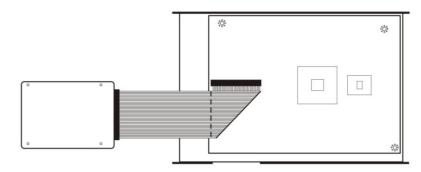
Step 5-1. HDD installation: Connect the HDD to IDE connector via HDD cable. Diagonally fold HDD-cable, as shown above.
