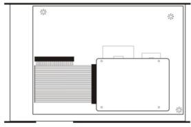
Step 5-2. Re-fold HDD cable as shown above for a proper installation of the HDD.
