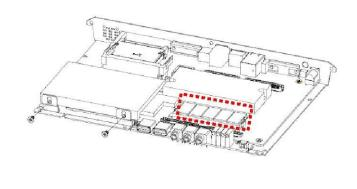
Step 4. Install the DDR SODIMM into the memory socket.
