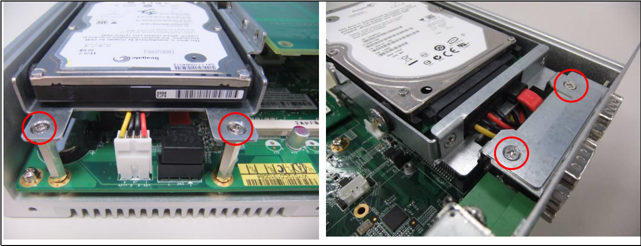
Fig. 6-6 Fasten HDD bracket with four screws.
