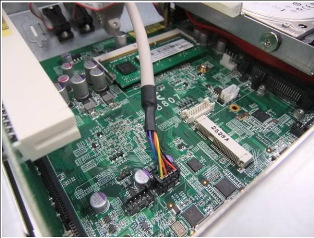
Fig. 9-1 Plug USB cable onto the motherboard.
