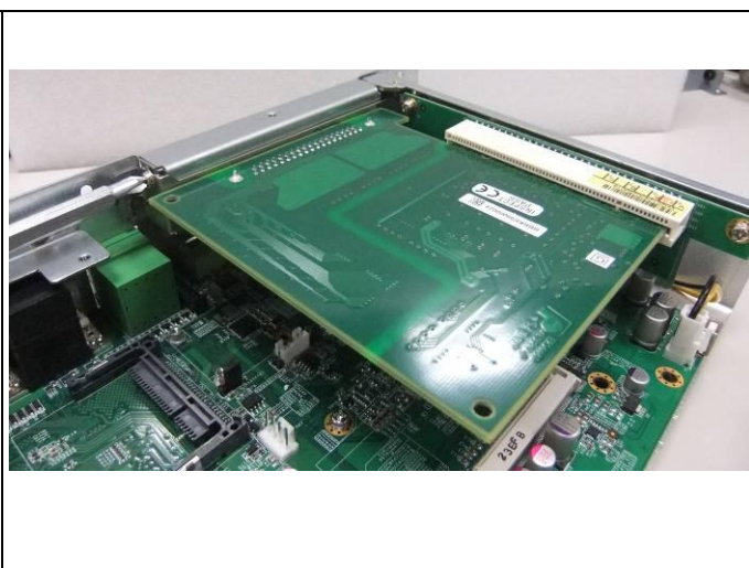
Fig. 11-4 Insert add-on card and fasten the screw.
