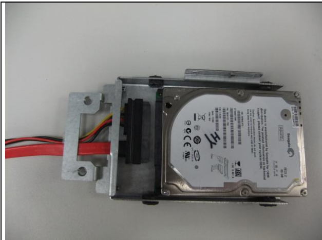
Fig. 6-3 Put HDD on the bracket
