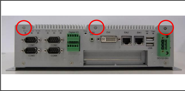
Fig. 4-1 Loosen three #6-32 screws on front panel.
