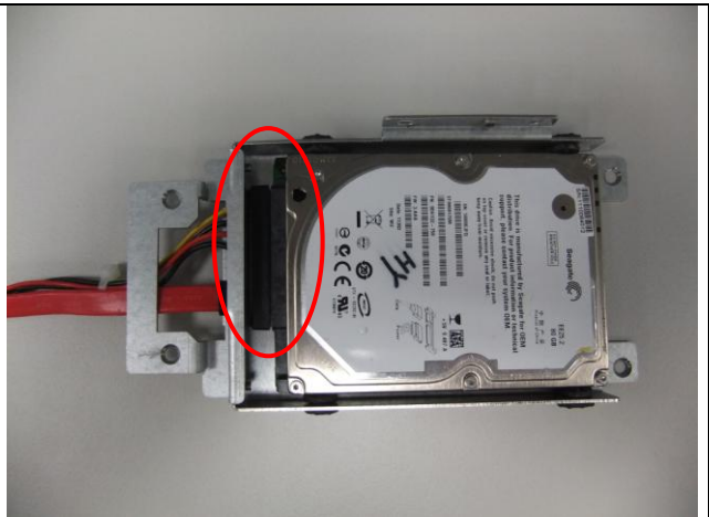
Fig. 6-4 Assemble cable and HDD
