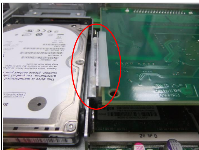
Fig. 11-5 Assemble HDD and make sure the guide rail fits the add-on card.
