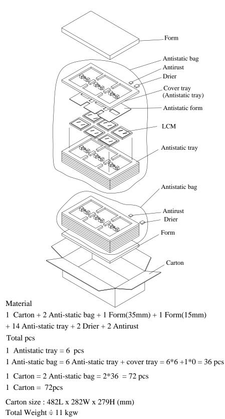
FG050722 TFT LCM PACKING
